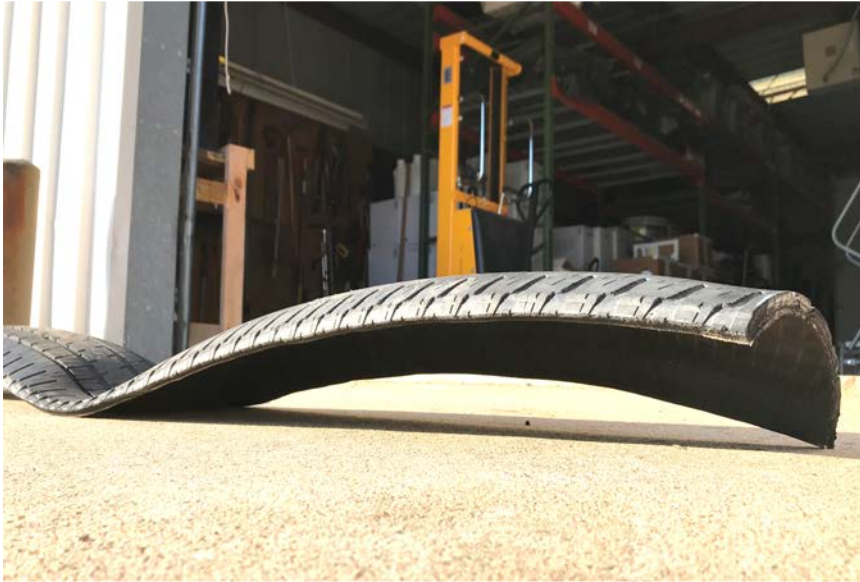
Section of tread exhibiting severe cupping.
