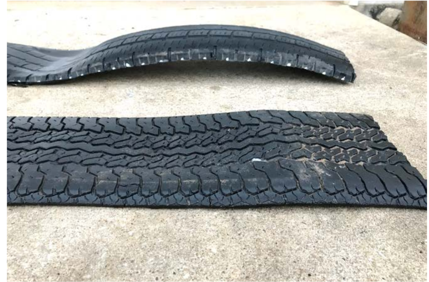
The lower (flat) section of tread is preferred because it presents less issues during lumber fabrication.
